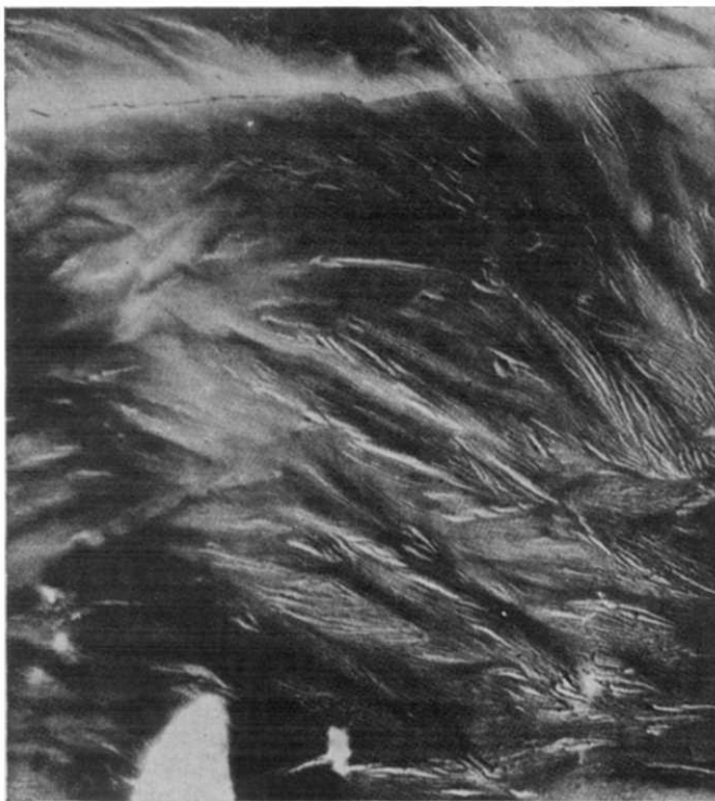
Figure 14 — \beta -Spherulite crystallized at about 130°C between slides (magnification \times 12\,500 ; reduced 2/3 on reproduction)
