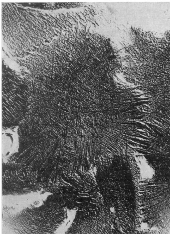
Figure 11 —Quadrites in polypropylene nucleated by 0.5 p.h.r. \text{AlOH}(\text{ptbb})_2 and crystallized at 143^\circ\text{C} with free surface (magnification \times 25\,000 ; reduced 2/3 on reproduction)
