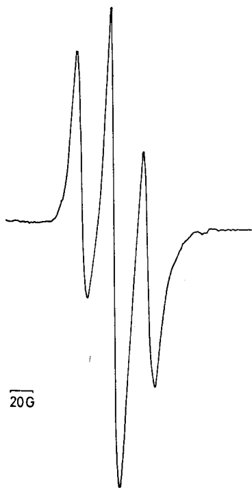
Figure 2 —The e.s.r. spectrum recorded at 77°K of 4-PVP irradiated at 77°K + 5 wt % \text{CHBr}_3
