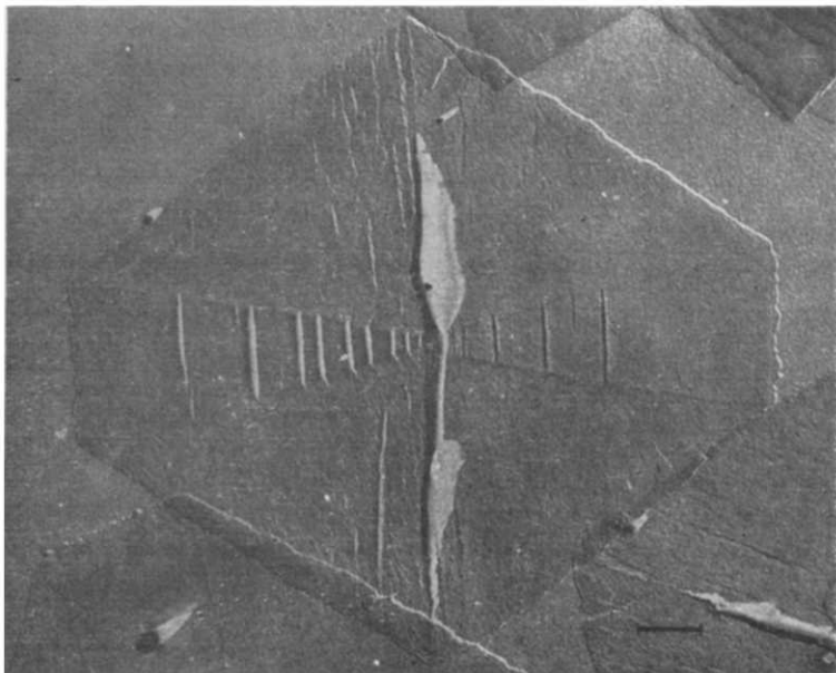
Figure 2 —Sample of Xy-87 crystals (annealed at 93^\circ\text{C} for 60 min) shows the representative crystalline morphology grown from xylene solution. The striations developed near the sector boundaries between the \{110\} sectors are only observed for annealed crystals
