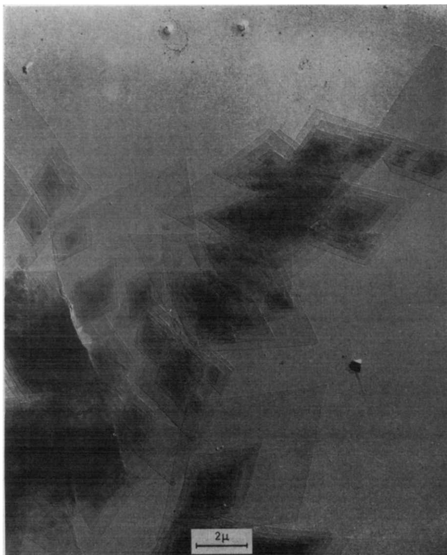
Figure 6 —Electron micrograph of slow cooled crystallized polyethylene (Alathon 71 X-N)
